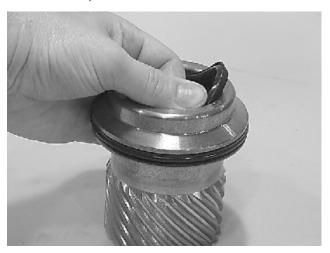
Beginning with the inner seal (200) insert one end of b/u ring in the lower groove and feed the rest in using a circular motion. Make sure the wedged ends overlap correctly.
