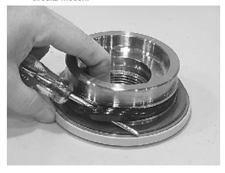
5. Install the wear guide (302) on the end cap (4) and shaft (2).
