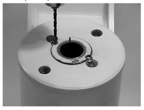
**3.** Remove the lock pins using an "Easy Out" (a size #2 is shown).
