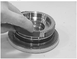
**6.** Install the inner T-seal (200) into the piston (3) using a circular motion.
