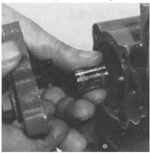
4. Re-install the bolts and tighten until the servo cover on the neutral adjustment side of the pump separates 0.125 in. (3 mm) from the housing. Turn the cover and remove and inspect the orifice.
