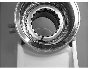
**12.** To remove the piston (3) use a rubber mallet and a plastic mandrel so the piston is not damaged.
