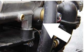
**NOTE:** Have a small container ready to collect oil that will drain freely from the regulator at this point.
