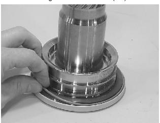
**4.** Using a seal tool install the main pressure seal (205) onto shaft (2) and end cap (4). Use the seal tool in a circular motion.
