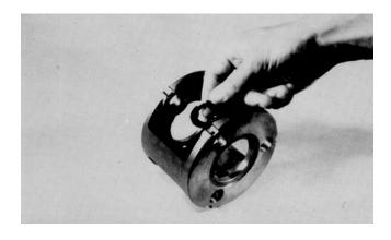
**6.** While keeping thrust washers in place, slide cluster gear into carrier with the larger gear on the side with the small pin hole.
