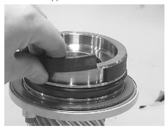
**16.** To remove the main pressure seals (205), it is easiest to cut them using a sharp razor blade being careful not to damage the seal groove.
