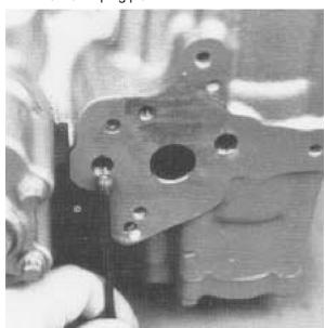
9. Align the control sleeve so its slot will engage the swash plate feedback pin (slot positioned toward the pump cover) and insert the sleeve into the housing. Carefully align the control spool with the sleeve and install the control onto the pump housing. Install the four mounting screws and torque to 10 to 11 ft.lbs. (13 to 14 Nm).
