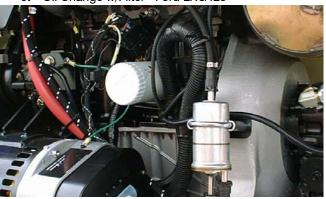
Lube Point(s) - Fill Cap/Spin-on Element
