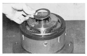
**11.** Place O-ring (5) into cover (6) counterbore. Use petroleum jelly to hold O-ring in place.
