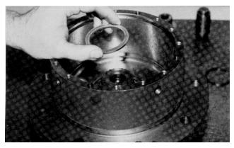
Retaining ring (1I) installed into groove provided in the output shaft (1A). This retaining ring (1I) should never be reused in a repair or rebuild.
