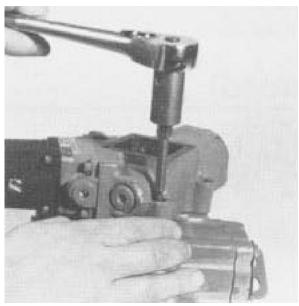
Carefully lift the control off the pump housing.
