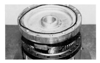
12. THe cover (6) is now installed on this assembly. Taking care to correctly align pipe plug hole (20) with those in the hub (1J), usually 90° to one another. Locate the 4 counterbore holes in hub (1G) (marked in step 3) and install 4 shoulder bolts (13). A slight tap with a hammer may be necessary to align shoulder bolt with hub (1G) counterbore.
