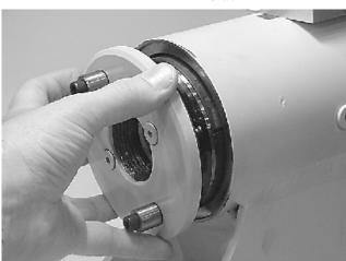
**17.** Tighten the end cap (4). In most cases the original holes for the lock pins will line up.
