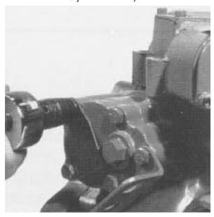
2. With a 7/32" internal wrench, remove and inspect the orifice.
