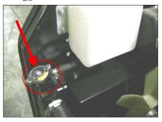
With the radiator cap still removed, start the engine and run until the thermostat opens. The thermostat opens at 170° F (77° C), which can be checked using the JLG handheld analyzer.
