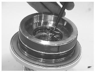
**15.** Remove the wear guides (302) from the end cap (4) and shaft (2).
