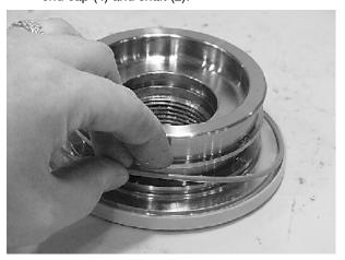
19. Remove the piston O.D. seal (202).
