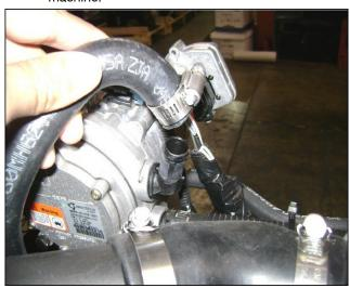
Remove the radiator cap. Fill the radiator with coolant until coolant starts to appear from the previously removed hose at the EPR. Reinstall the hose back onto the EPR and continue to fill radiator with coolant
