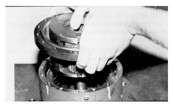
**NOTE:** If gears do not mesh easily or carrier assembly does not rotate freely, then remove the carrier and ring gear and check the cluster gear timing.
