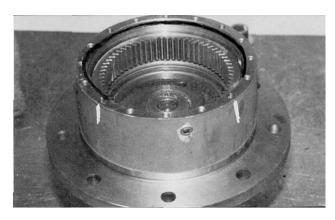
4. Thrust spacer (9) is installed into the bore of the output shaft (1A). This should be a slip fit and thrust spaces should rotate in this location.
