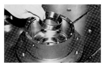
4. Returning the hub (1G) to locate on the large diameter end, the output shaft (1A) is carefully installed into the hub (1G).
