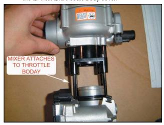
**4.** Place gasket on intake manifold and attach mixer/ throttle assembly to manifold.
