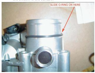
2. Install the two quad seals. Install one seal at a time to insure the seal does not roll. The seal must sit flat on the throttle body.
