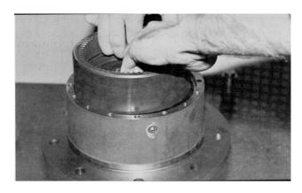
2. Thrust washer (11) is installed on the face of the output shaft (1A). Sufficient grease or petroleum jelly should be used to hold thrust washer in place.
