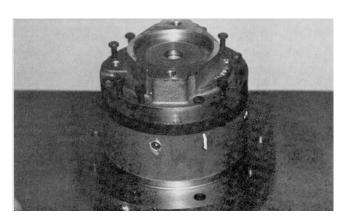
**14.** Pipe plugs (20) are to be installed into cover (6) using a lubricant of some sort.
