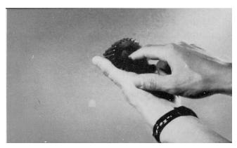
2. Place sixteen needle rollers into cluster gear bore.
